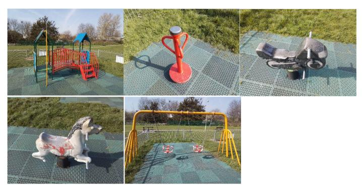
The toddler area contains a multi-play unit, low rotator, spring motorbike, spring horse and a swing set. The equipment was installed several years ago but is still in good condition, with the main issues picked up on the last inspection being worn paintwork, surface corrosion and rust, which are all treatable. The site was assessed as 'low risk' overall. The play surfacing was replaced with 'Matta' surfacing in 2022 and therefore requires no maintenance work at this stage.
